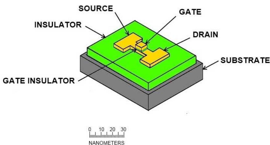
**Left:** The new Avto Quantum Transistor comprises a metallic thin-film with source and drain, beneath a several Å-thick gate insulating layer and gate.
